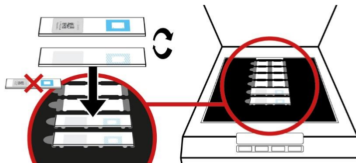
Figure 4: loading of VisionArray Chips in the slide holder of the Scanner V600 Photo
